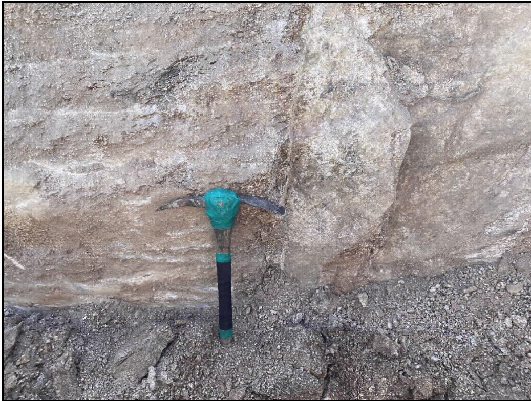
Figure 3-4. Test Pit, TP-1, Exposing Val Verde Tonalite
