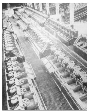
**Figure 18.** Flotation Section at Pine Creek uses M.S. machines, makes copper, molybdenum, and scheelite concentrate (Photograph from *Engineering and Mining Journal*, May 1951:83.)
