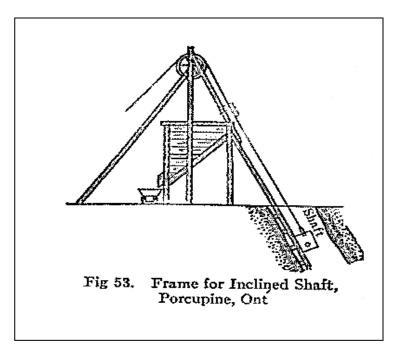
**Figure 36.** Diagram of an A-frame headframe for an inclined shaft from Peele's *Mining Engineers' Handbook*, published in 1927 (Peele 1927: 1091).
