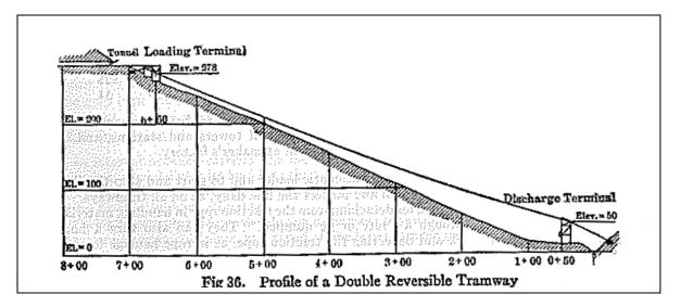
Figure 37. Diagram of Double Reversible Tramway Used for Mining Ores (Peele 1927:1784).
