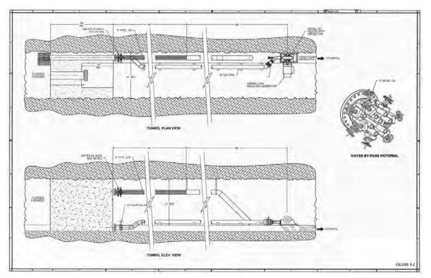
Figure 5. Plan view of Adit Plug.
