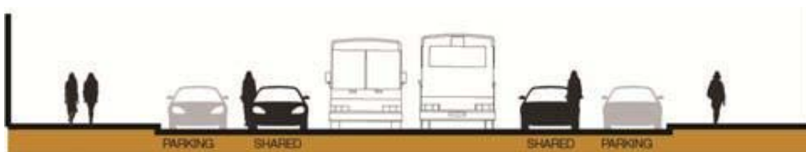
Figure 6. Mission Street Alternative with Center-running Bus Lanes. Bus lanes would be 13 feet wide, the outer lanes would be 13 feet, 3 inches wide. The illustration shows the condition outside of the Sixth Street to Fremont Street corridor (within which there would be no space for parking).
