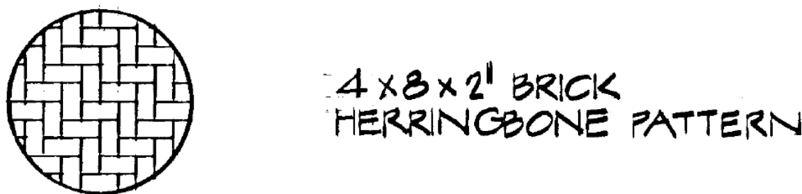
Figure 4. From Contract Drawings for Market Street Reconstruction: Herringbone Brick Pattern
