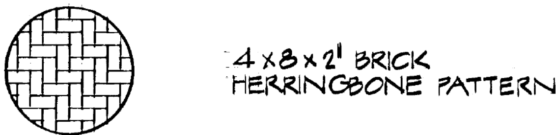
Figure 1-5. From Contract Drawings for Market Street Reconstruction: Herringbone Brick Pattern
