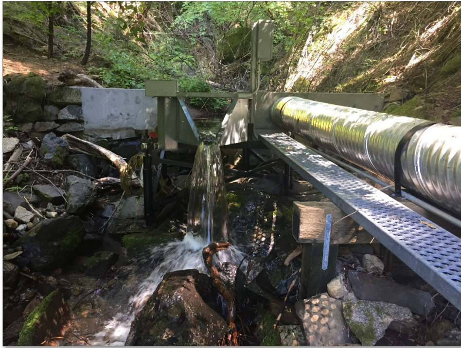
Bull Creek streamguage and diversion pipe.
