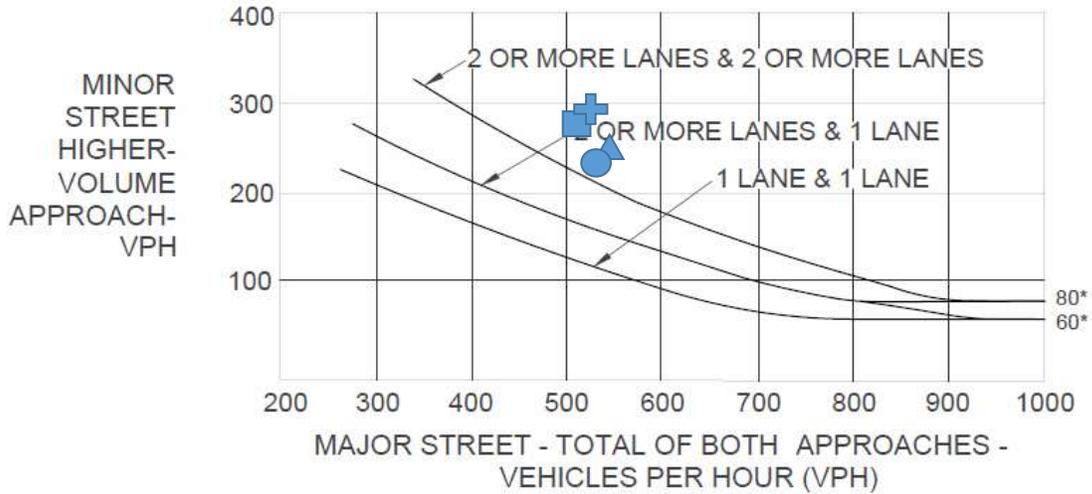
\*Note: 80 vph applies as the lower threshold volume for a minor-street approach with two or more lanes and 60 vph applies as the lower threshold volume for a minor street approach with one lane.
