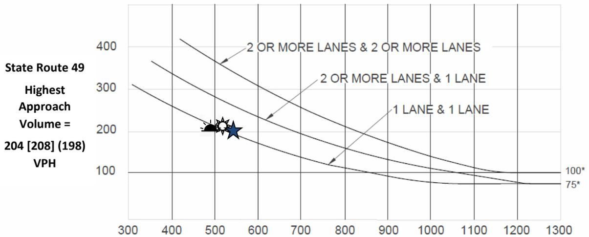
\*Note: 100 vph applies as the lower threshold volume for a minor-street approach with two or more lanes and 75 vph applies as the lower threshold volume for a minor street approach with one lane.
