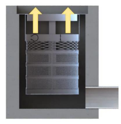
Remove the hydrocarbon boom that is attached to the inside of the filter basket. The hydrocarbon boom is zip tied to the top perimeter of the filter. Assess the color and condition of the boom using the following information in the next bullet point. If replacement is required, install and fasten on a new hydrocarbon boom.
