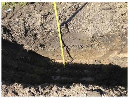
Figure 7: Trench 4 soil profile, north/northwest sidewall, measuring at 120cm depth.
