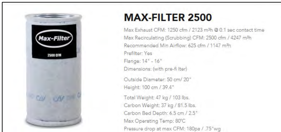
Figure 2. The above depiction is an example of a carbon filter that, when used in conjunction with a fan as shown in Figure 1 above, neutralizes odors.
