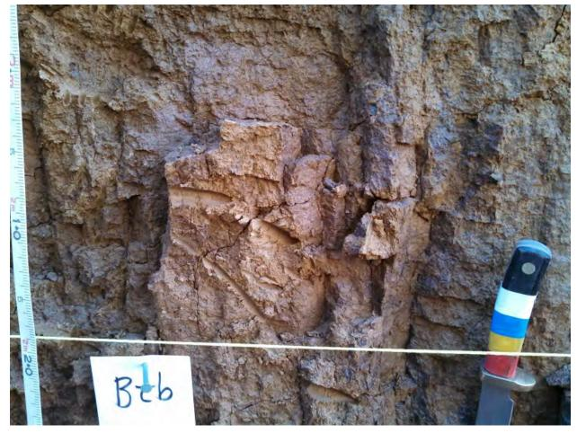
Figure 6. Close up of the Btb of the Early Wisconsin paleosol in Soil Profile No. 6. Note the silvery mangans above the knife handle. View SE.
