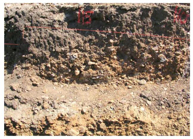
Figure 11. Early Wisconsin paleosol uplifted against the northeastern side of the pressure ridge in the vicinity of stations 0+10 and 0+15. Elsewhere, this weathered cobble of the San Benito Formation is at least 160 cm beneath the surface. View SE.
