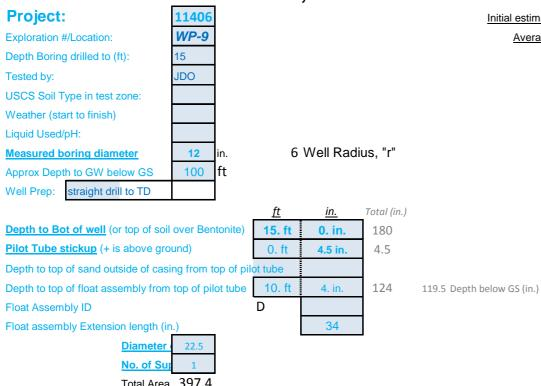
Initial estimated Depth to Water Surface (in.): 152.83 Average depth of water in well, "h" (in.): 27.169 approx. h/r: 4.5 Tu (Fig. 8): 87.3 ft
