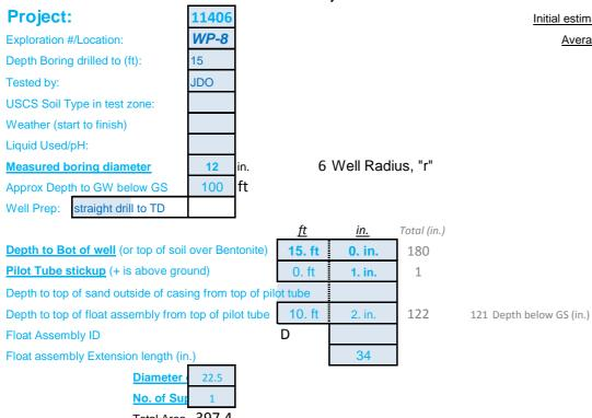
Initial estimated Depth to Water Surface (in.): 141.38 Average depth of water in well, "h" (in.): 38.623 approx. h/r: 6.4 Tu (Fig. 8): 88.2 ft
