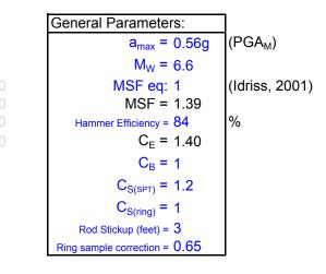
Summary of Liquefaction Susceptibility Analysis: SPT Method Liquefaction Method: Youd and Idriss (2001). Seismic Settlement Method: Tokimatsu and Seed (1987) and Martin and Lew (1999). Project: Stratham Rancho Cuamonga Project No.: 11406.001
