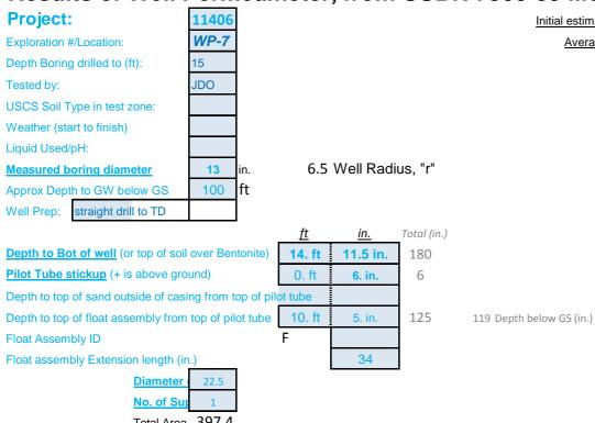
Initial estimated Depth to Water Surface (in.): 150.65 Average depth of water in well, "h" (in.): 28.848 approx. h/r: 4.4 Tu (Fig. 8): 87.4 ft Tu>3h?: yes, OK
