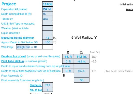
Initial estimated Depth to Water Surface (in.): 141.44 Average depth of water in well, "h" (in.): 38.058 approx. h/r: 6.3 Tu (Fig. 8): 88.2 ft
