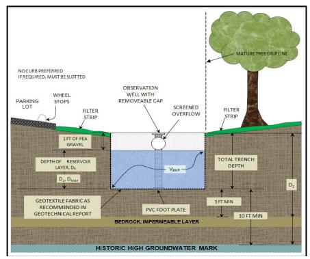
Figure 1 Section View of an Infiltration Trench
