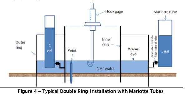
The purpose of the outer ring is to promote one-dimensional and vertical flow beneath the inner ring forcing the water contained in the inside ring to percolate straight downward and not to the sides. As rule of thumb, horizontal permeability is ten times greater than vertical permeability depending on the environment of deposition. By measuring the vertical permeability, we have determined the most conservative infiltration rate.
