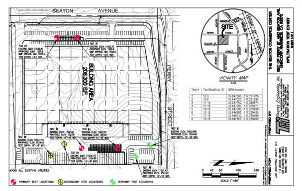
Figure 2 – Site Plan showing locations of tests
