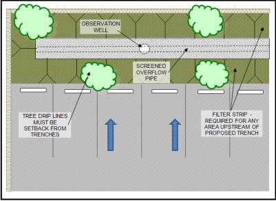
Figure 2 Plan View, Sheet Type Flows
