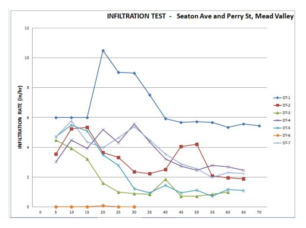
Figure 5 - Graphical Results of Double Ring Testing
