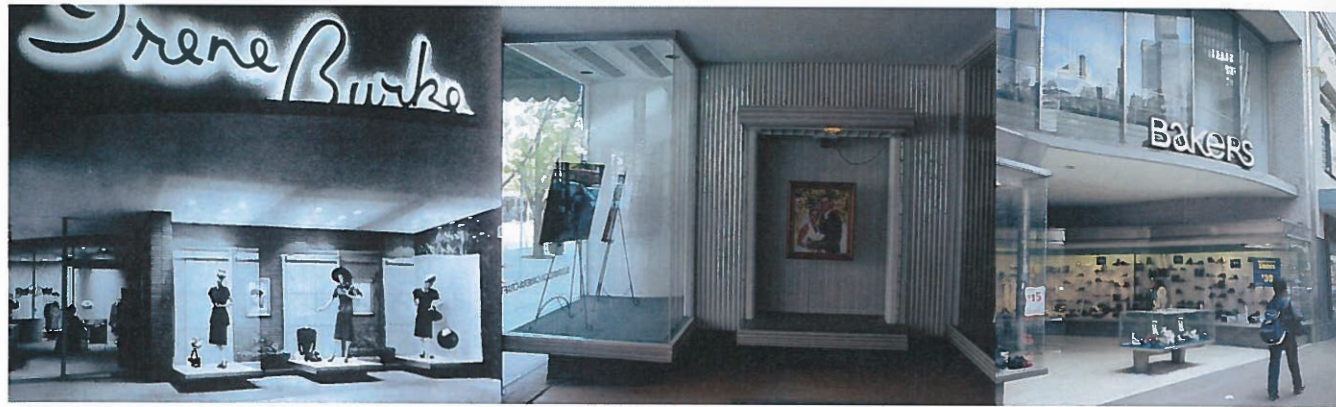
Figure 5: Cantilevered display cases in outdoor lobbies deconstructed the front plane of retail buildings. Left, a design in Long Beach, California, from Design for Modern Merchandizing , April 1948, p. 126. Center, similar displays in Bloomington, Illinois. Right, the former Bakers Shoes in Chicago, Illinois, had a free-standing display table, well lit cantilevered display cases and a curved open front display window on the second floor, photo: author. Center photo: IHPA archives.
