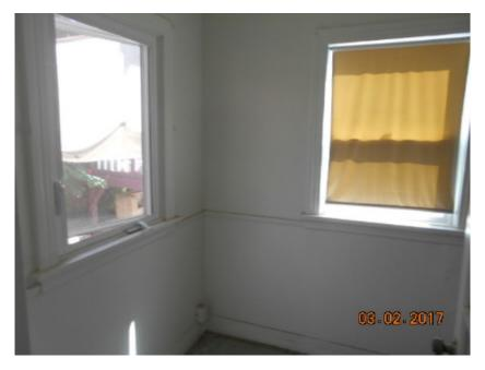
2. Typical bedroom. Interior perimeter walls, window frames and baseboard are covered with intact, undamaged, lead-containing paint.
