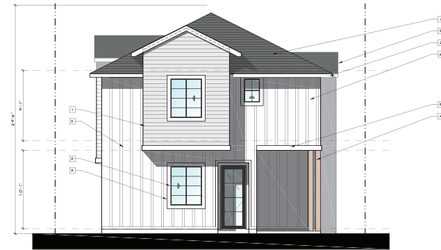
COTTAGE - EXTERIOR ELEVATIONS - 'B' 3/16"=1'-0"
