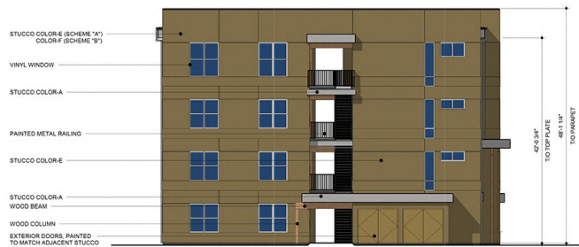
3 LEFT ELEVATION - BUILDING 1 3/32" = 1'-0"
