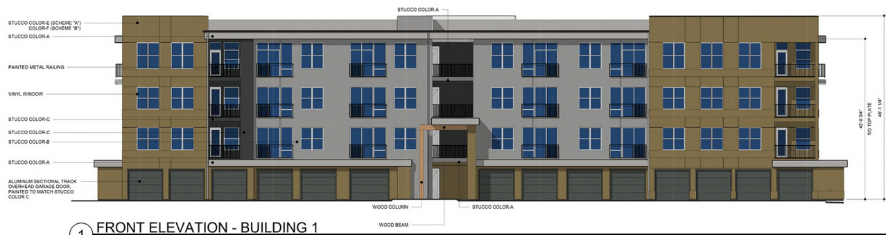
1 FRONT ELEVATION - BUILDING 1 3/32" = 1'-0"
