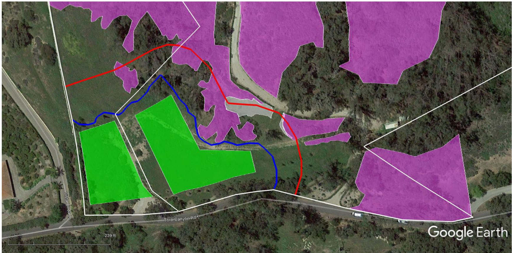
Figure 1. Revised ESH map based on conditions existing on 4 April 2019. Lot boundaries are shown by white lines (Lot 1 at left; Lot 2 at right); Building Envelopes are shown in green; Development Envelope boundaries are shown by blue line; 100-foot Fire Fuel Management limits from Building Envelopes is shown by red line. Vegetation: coastal sage scrub (ESH): purple; native grass concentrations (ESH): white; uncolored areas show non-native vegetation (ruderal, ornamental, eucalyptus-dominated woodland with scattered coast live oaks and a patchy understory of coastal sage scrub). Toro Canyon Road runs along bottom of image. North is to upper right. Imagery dated. 12 April 2018.
