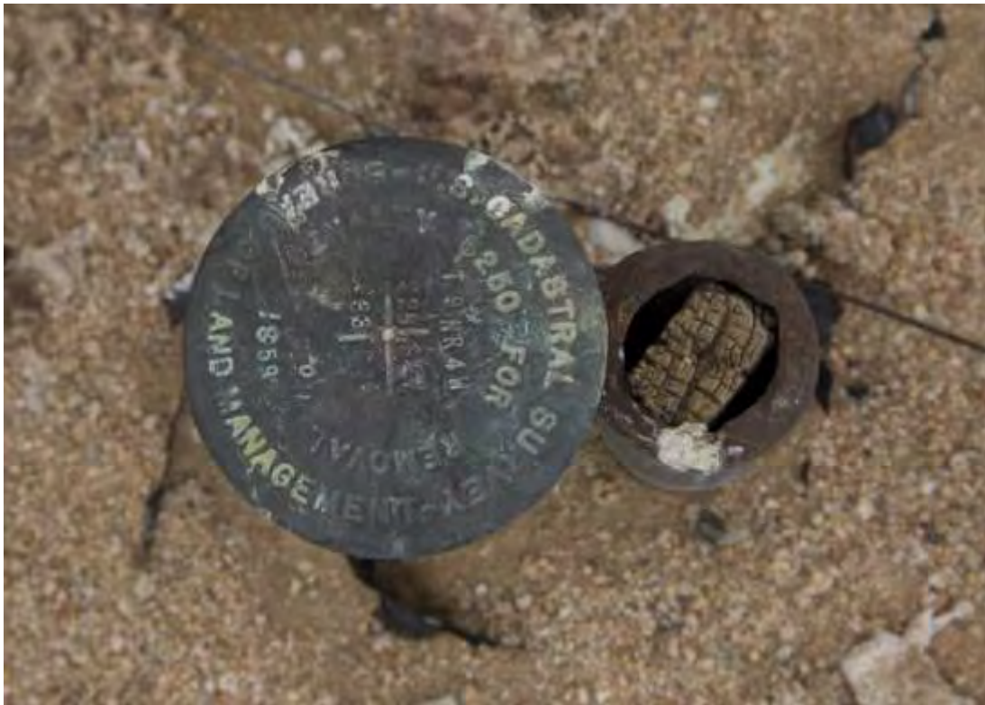
Figure 1. Top view of the Brass Disk of the U.S. Cadastral Survey marker.
