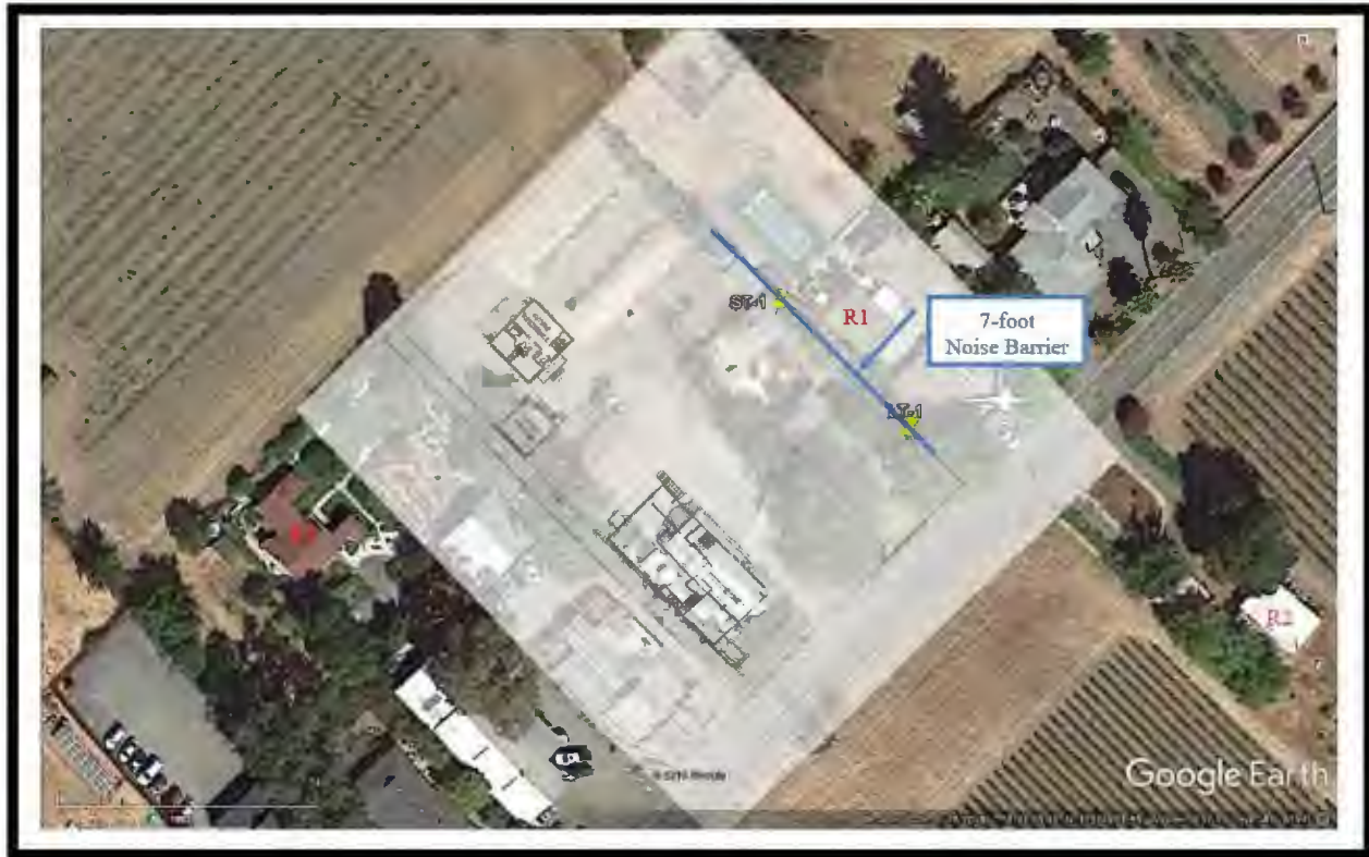
Figure 12. Additional noise attenuation fence on northeast property line. From Figure 2 of Illingworth & Rodkin, Inc. Noise Assessment. A minimum 7 foot high 185 foot long noise barrier, constructed along the northeast property line constructed solid over the face and base of barrier from materials with a minimum surface weight of 3 lbs per square foot (suitable materials include a 1 inch nominal thickness wood fence, masonry block, or concrete).
