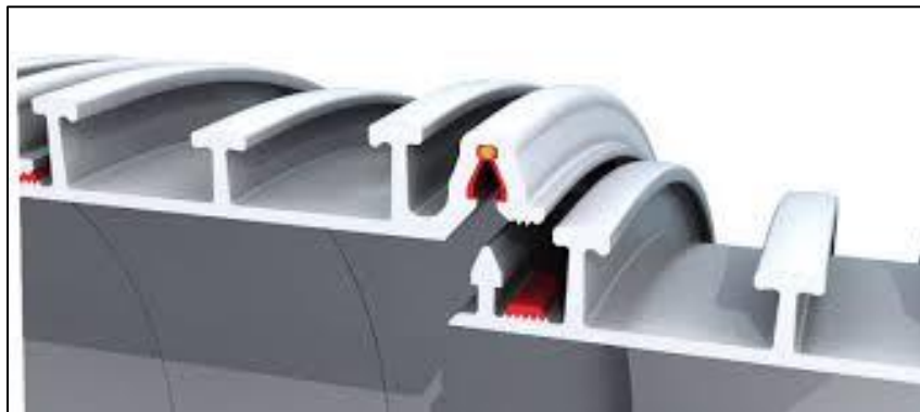
Figure 2-10: Interlocking Edges of PVC Profile Strip for Sekisui SPR™ TF Spiral Wound Liner
