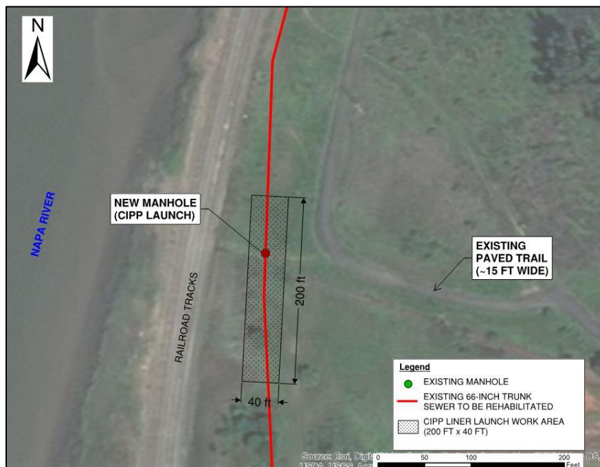
Figure 2-8: Potential CIPP Liner Launch Work Area Layout at the New Manhole
