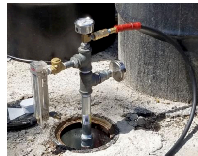
Typical pilot test air sparge injection into well.
