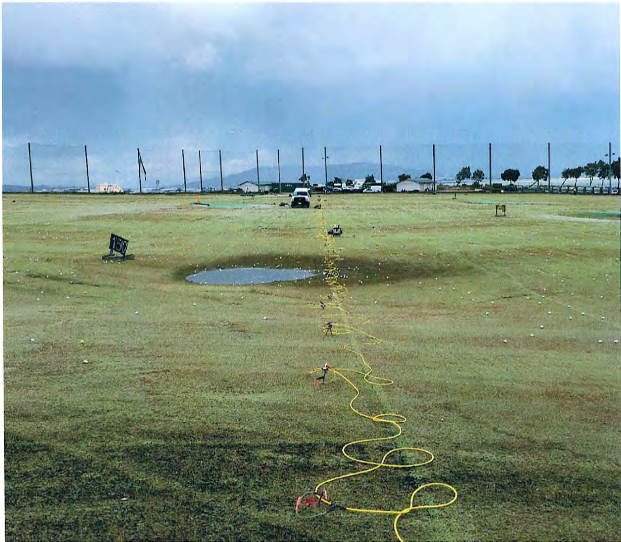
Figure 1: Driving range interior viewed from the southeast side looking northwest along Line 2. Resistivity cable (yellow) connects 56-electrodes (metal stakes) to instrumentation housed in the vehicle in the distance. The area with standing water is a surface depression that may be caused by a sinkhole.
