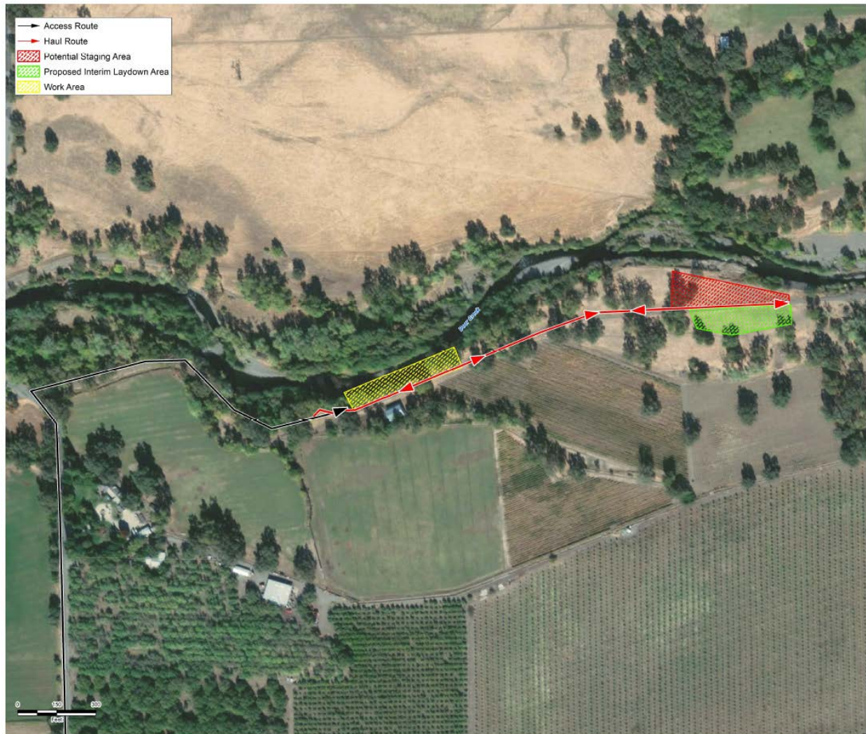
Figure 4. Proposed construction work area, staging and laydown areas, and haul and access routes for Site 80 erosion repair.
