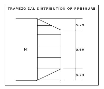
Where a combination of sloped embankment and shoring is utilized, the pressure will be greater and must be determined for each combination. Additional active pressures should be applied where the shoring will be surcharged by adjacent traffic or structures.
