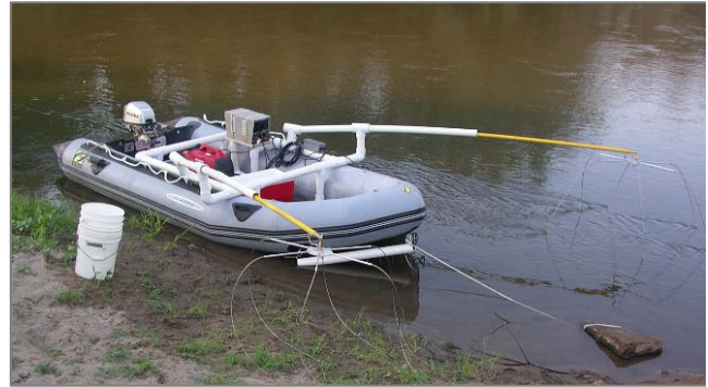
Figure 2-9 Photograph of Boat-Mounted Electrofishing Apparatus
