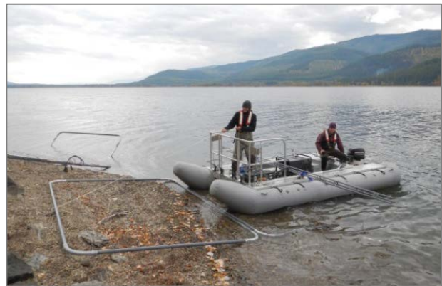
Figure 2-11 Photographic of Benthic Electrode Array being Prepared for Deployment
