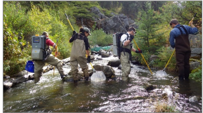
Figure 2-10 Photograph of Backpack Electrofishing in a Shallow Headwater Stream
