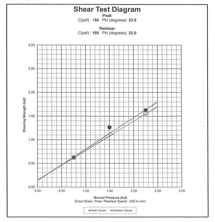
Sample Remolded to 90% Relative Density, saturated. Remolded Dry Density = 115.7 PCF
