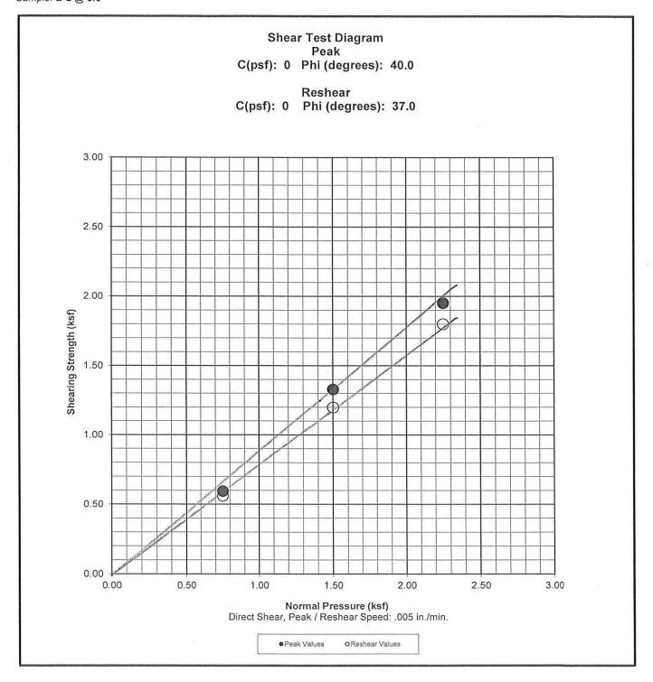
Undisturbed Natural Shear-Saturated
