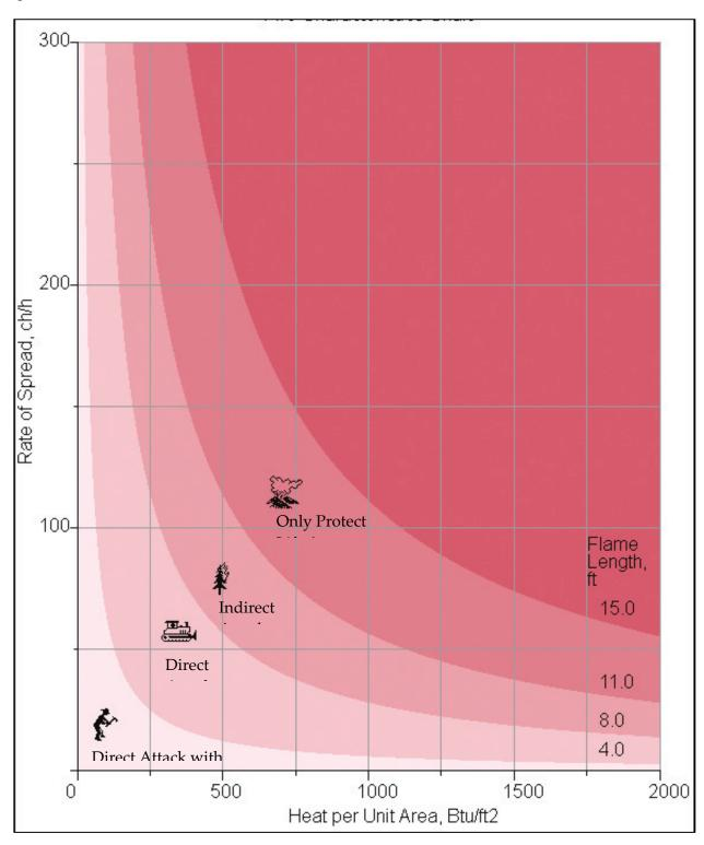
Figure 16 Surface Fire Behavior Fire Characteristics Chart
