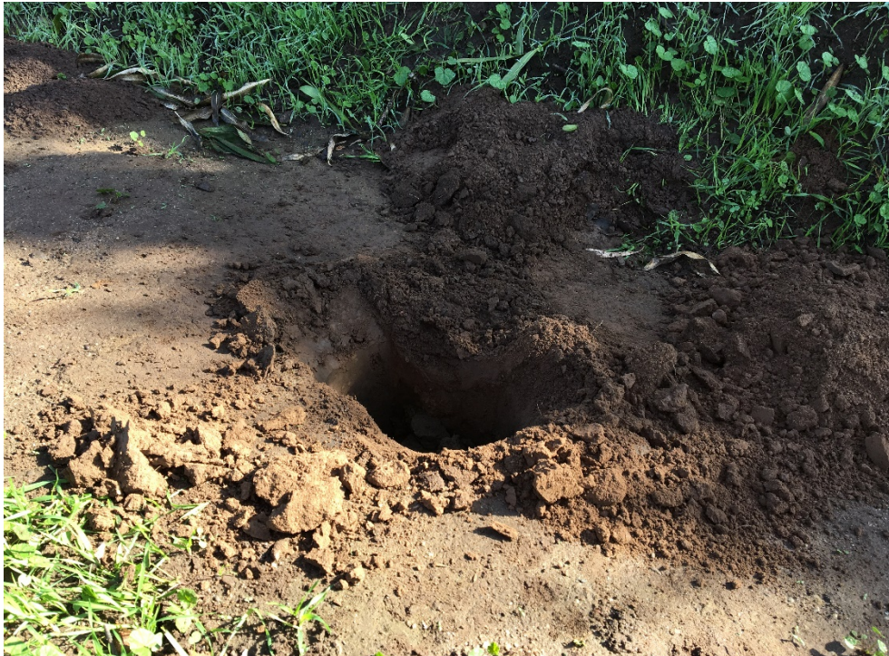
Ditch 1 – Soil Test Pit 1. Note: silty sand substrate at this location.
