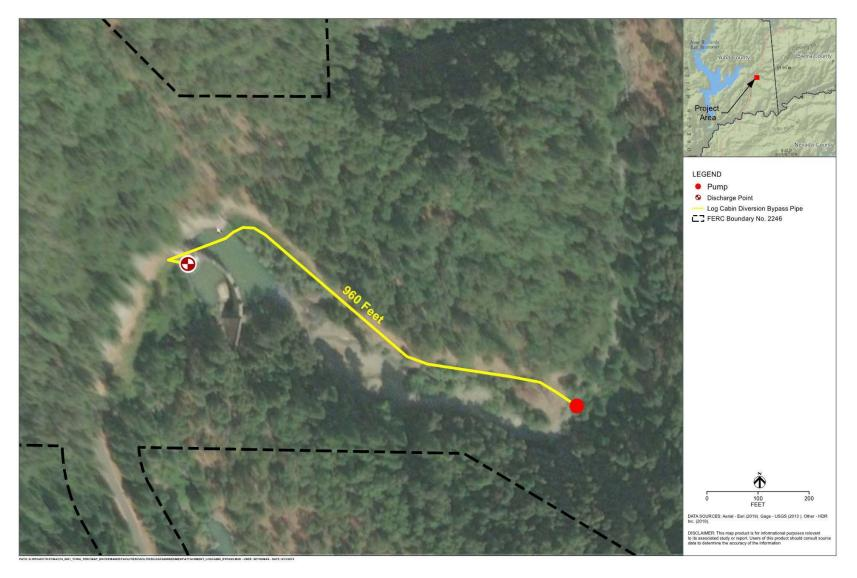
Figure 2.3-3. Proposed layout of pumps and pipes for the diversion at Log Cabin Diversion Dam.
