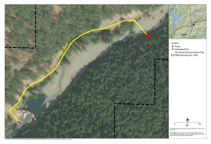
Figure 2.3-2. Proposed layout of pumps and pipes for the diversion at Our House Diversion Dam.
