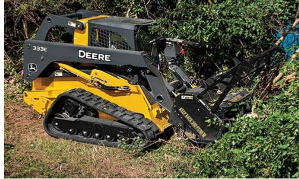
**Photo 2.** Skid steer with masticating/mulching attachment.
