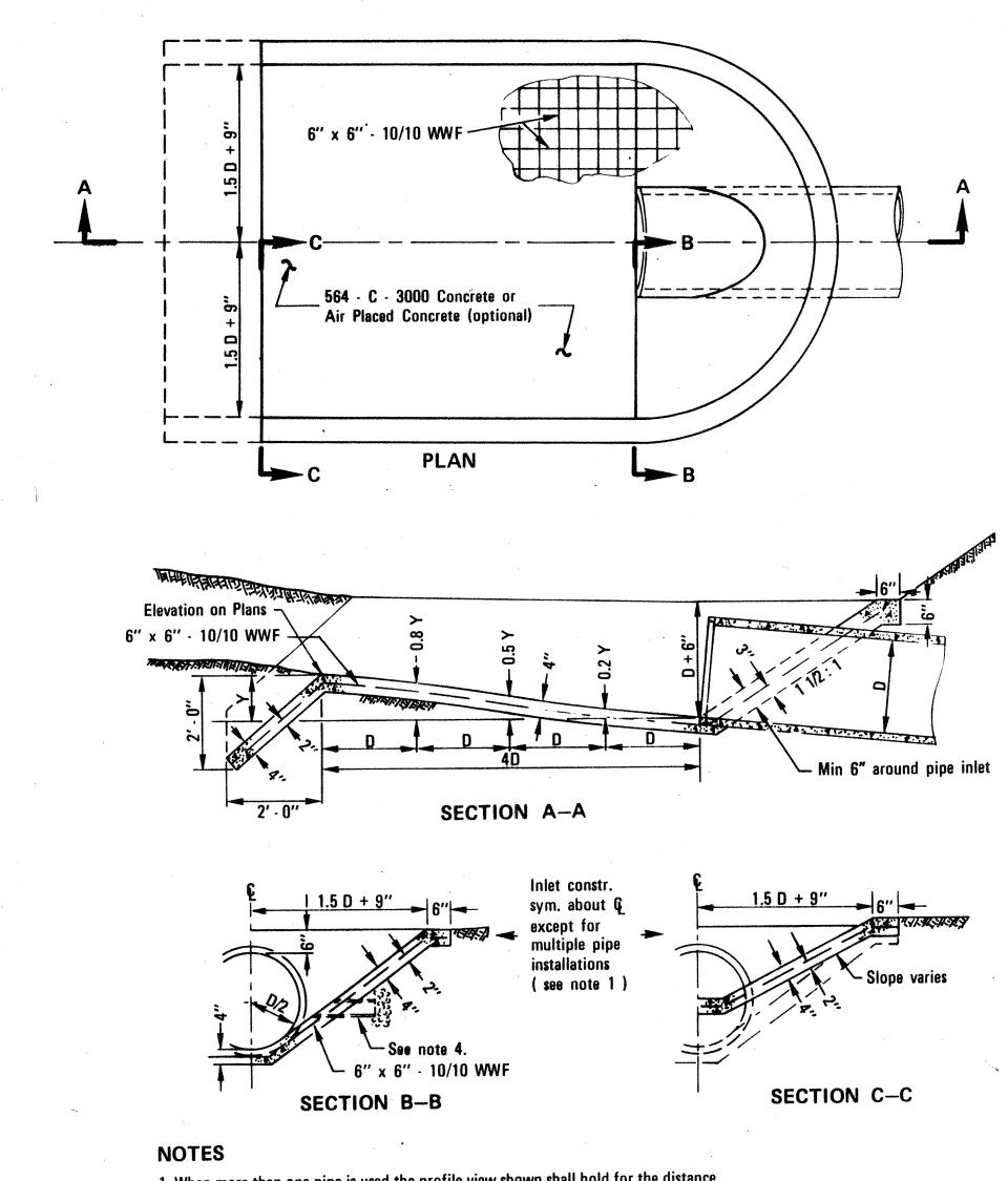
1. When more than one pipe is used the profile view shown shall hold for the distance across all pipe openings. Sections A-A and B-B shall be from the outermost pipe. The
