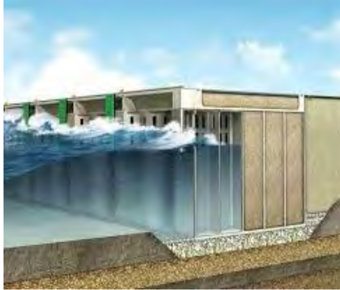
Figure 5-5: Example of multi-chamber perforated caisson structure, Ko et. al. (2009)
