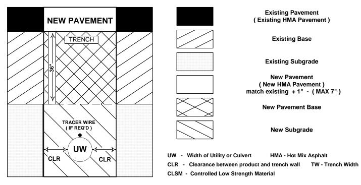
STRUCTURE BACKFILL SHALL CONFORM TO SECTION 19 - 3.06 OF THE STANDARD SPECIFICATIONS
