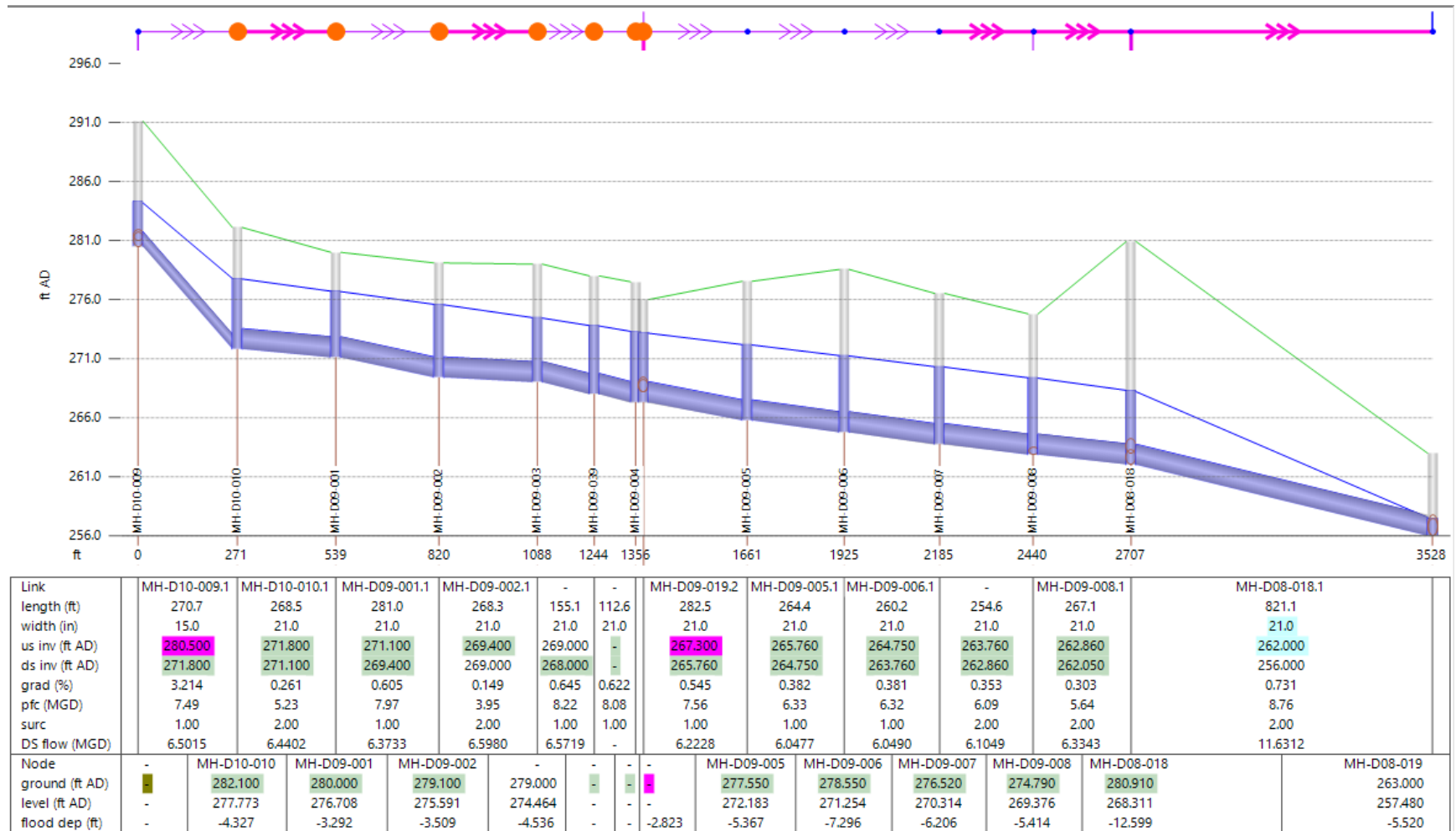
Figure 5: Model Profile of Downstream 21-inch Sewer MH-D10-009 to MH-D08-019
