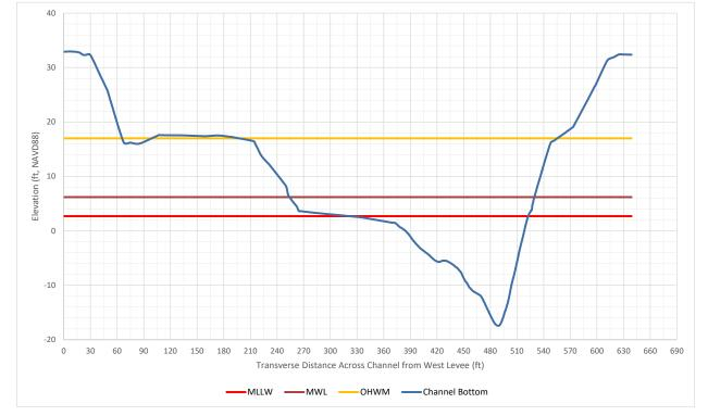
Figure 2. San Joaquin River channel cross-section at proposed outfall location, with the mean lower low water (MLLW) level, mean water level (MWL), and ordinary high water mark (OHWM) shown.
