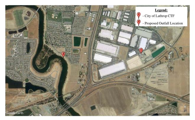
Figure 1. Map of City of Lathrop CTF and proposed San Joaquin River discharge outfall location.
