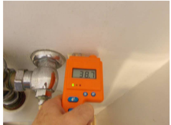
DSCN26891 st Fl Bathroom, Confirmation Area (Wet), Hard to Touch or Penetrate with Pins
