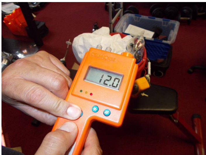
DSCN2653 Calibration/Battery Good when 12.0 is Displayed
