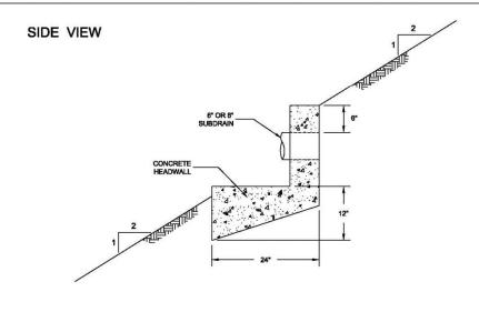
NOTE: HEADWALL SHOULD OUTLET AT TOE OF FILL SLOPE OR INTO CONTROLLED SURFACE DRAINAGE
