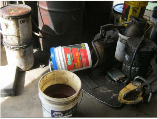
Photo # 11: showing hazardous waste area with no Aisle Space and Waste Oil drums not Labeled
