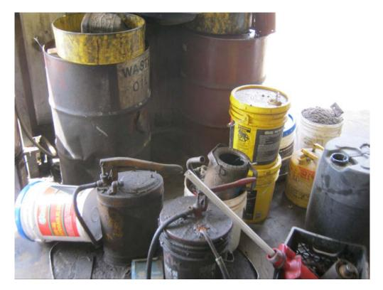
Photo # 12: showing hazardous waste area and Waste Oil drums not Labaled
