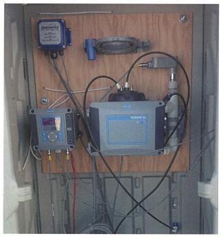
Figure 4-1. Example of EC and Turbidity Instruments used in Pilot Study
