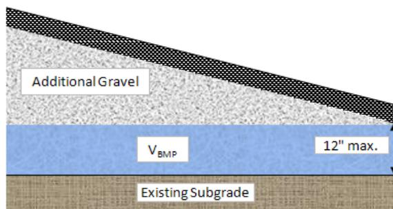
**Figure 3: Sloped Cross Sections for Permeable Pavement**
