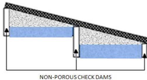
**Figure 4: Permeable Pavement with Non-permeable Check Dams**
