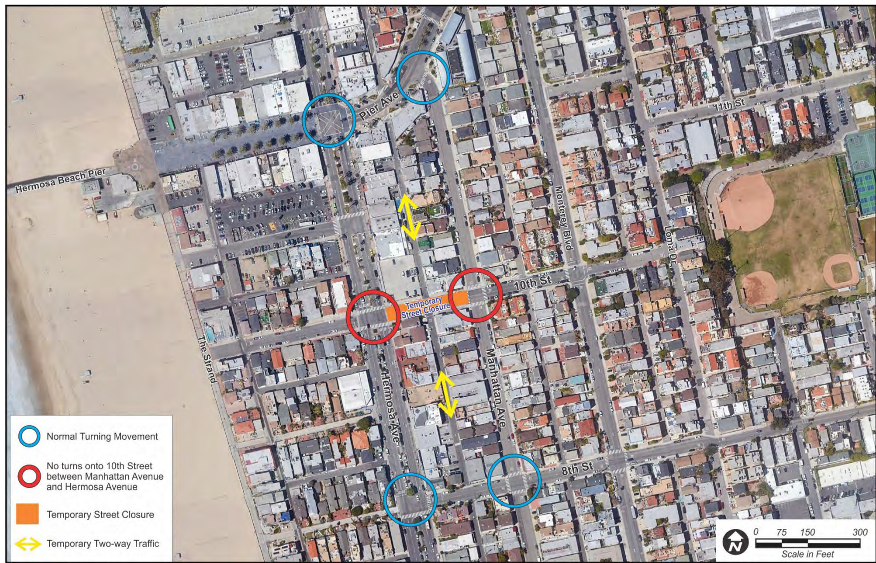
Figure 3.11-2. Temporary Traffic Changes at the Proposed 10th Street Cable Landing Site
