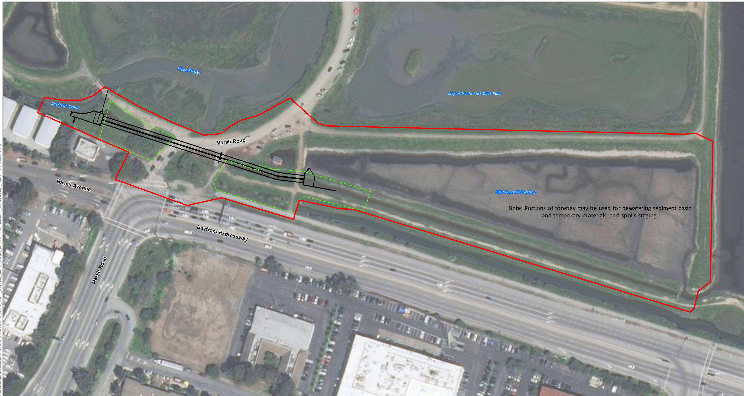
Figure 6 Construction Plan Access, Staging, and Dewatering
