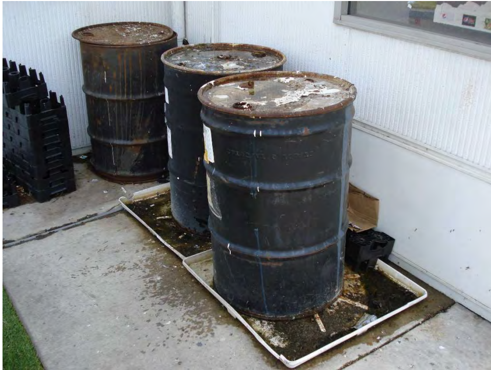
Photo 27 – View of Mobil (3909 Hallmark Parkway) facing north. Three 55-gallon metal corroded drums are stored behind the car wash facility. The hazardous material label on the second drum stated oil and gasoline are stored in the drum. De minimis staining was observed on the surface of the underlying concrete beneath the drums.
