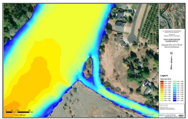
Figure 9. SRH2D Velocity results for proposed conditions
