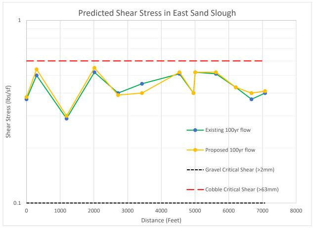
Figure 4. Hec-RAS Shear Stress results
