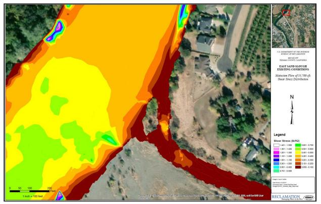
Figure 6. SRH2D Shear Stress results for existing conditions
