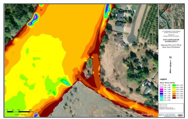
Figure 7. SRH2D Shear Stress results for proposed conditions
