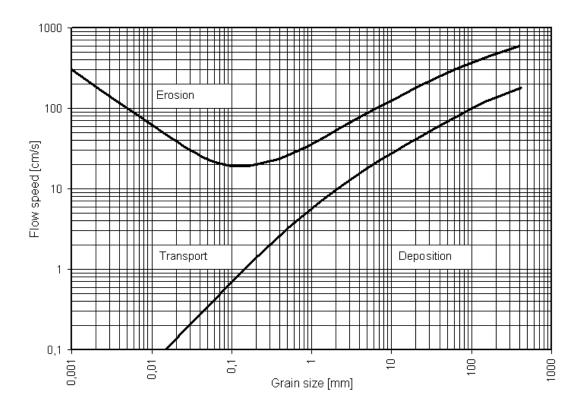
Figure 5. Hjulstrom Curve
