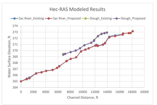
Figure 3. Hec-RAS Proposed design modeled results
