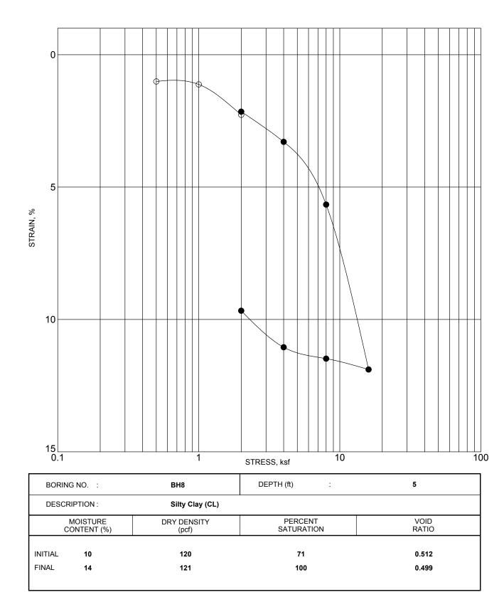
NOTE: SOLID CIRCLES INDICATE READINGS AFTER ADDITION OF WATER
