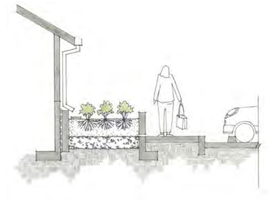
Bioretention facility adjacent to building. An impermeable cutoff wall between the facility and the building may be incorporated.
