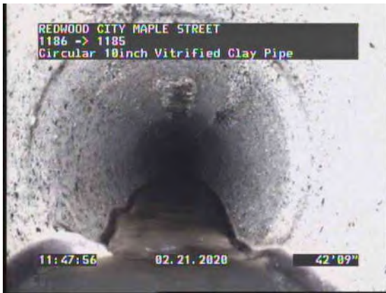
13, 00:06:13, 42.79ft Lining Failure Bulges from 7 o'clock to 8 o'clock, within 8 inch
