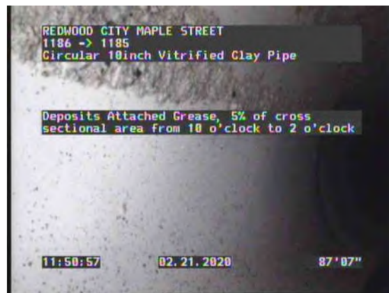
16, 00:09:10, 87.58ft Deposits Attached Grease, 5% of cross sectional area from 10 o'clock to 2 o'clock
