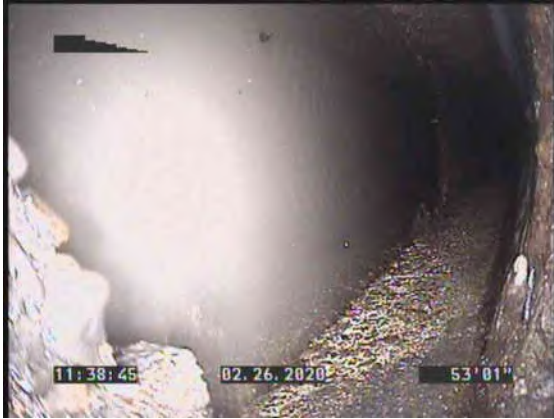
13, 00:05:00, 53.06ft Survey Abandoned / JOINT OFFSET LARGE
