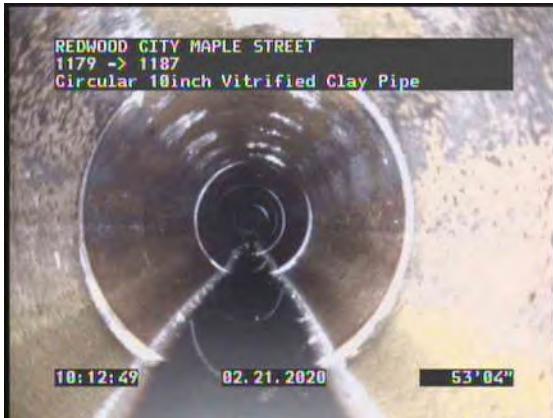
17, 00:06:09, 53.36ft Water Level, Sag in pipe, 15% of the vertical dimension
