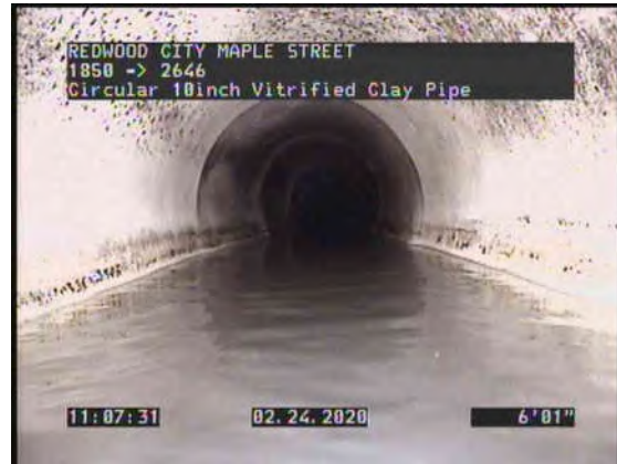
6, 00:01:19, 5.89ft Water Level, Sag in pipe, 35% of the vertical dimension
