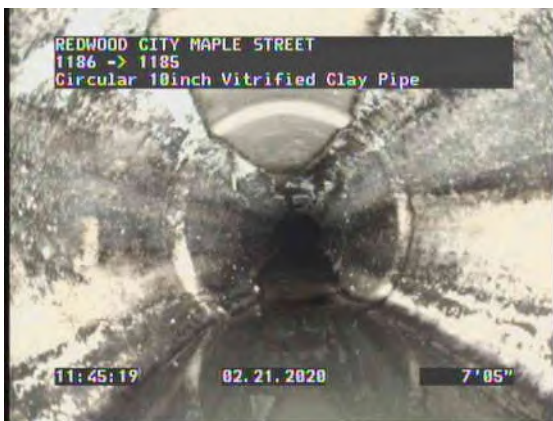
7, 00:03:59, 7.38ft Deposits Attached Other, 5% of cross sectional area from 8 o'clock to 4 o'clock, Start
