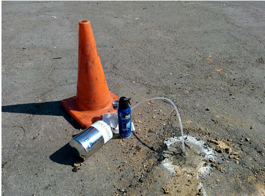
Subject: Soil gas sample collection using Difluorochloroethane (DFA) as a leak detection compound.
