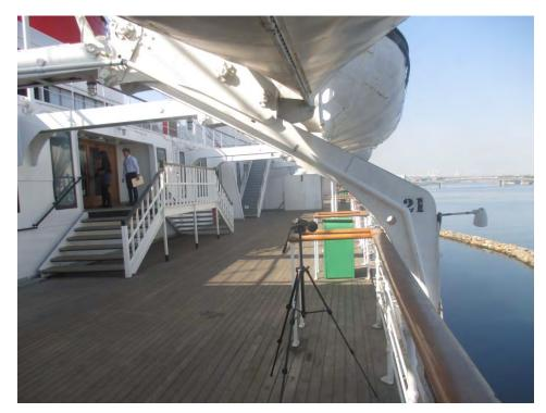
Photo 5: Airborne Sound Monitoring Location (ST3; short-term station) for Long Beach Cruise Terminal.
