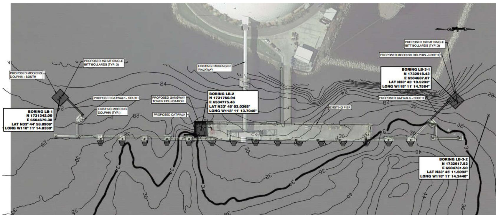
Figure 1. Boring locations for structural elements at the Long Beach Cruise Terminal
