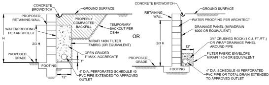
Typical Retaining Wall Drainage Detail
