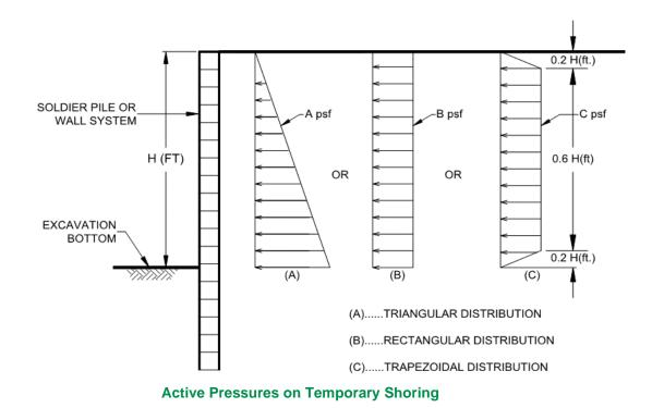
7.5.8 The passive resistance can be assumed to act over a width of three pile diameters. Typically, soldier piles are embedded a minimum of 0.5 times the maximum height of the excavation (this depth is to include footing excavations) if tieback anchors are not employed. The project structural engineer should determine the actual embedment depth.
