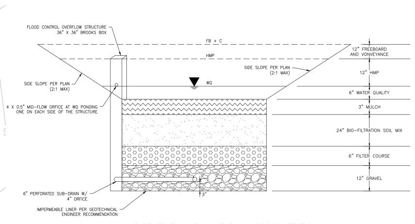
BIOFILTRATION BASIN TYPICAL CROSS SECTION NOT TO SCALE
