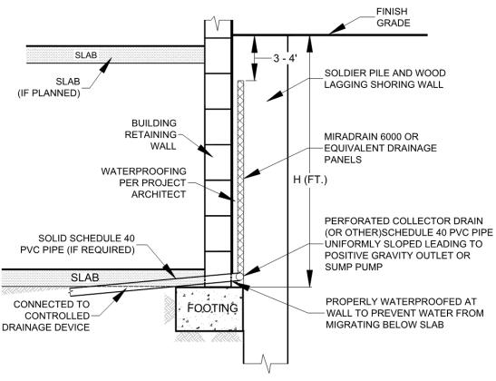
Shoring Retaining Wall Drainage Detail
